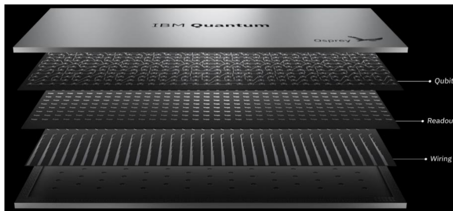
Image 2. The Three Fundamental Layers of Superchips: Qubit, Readout, Wiring. Source:
