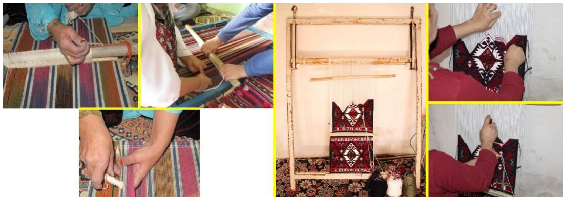
Illustration 14: Plain Weave and Kilim (Flat-Weave) Technique
